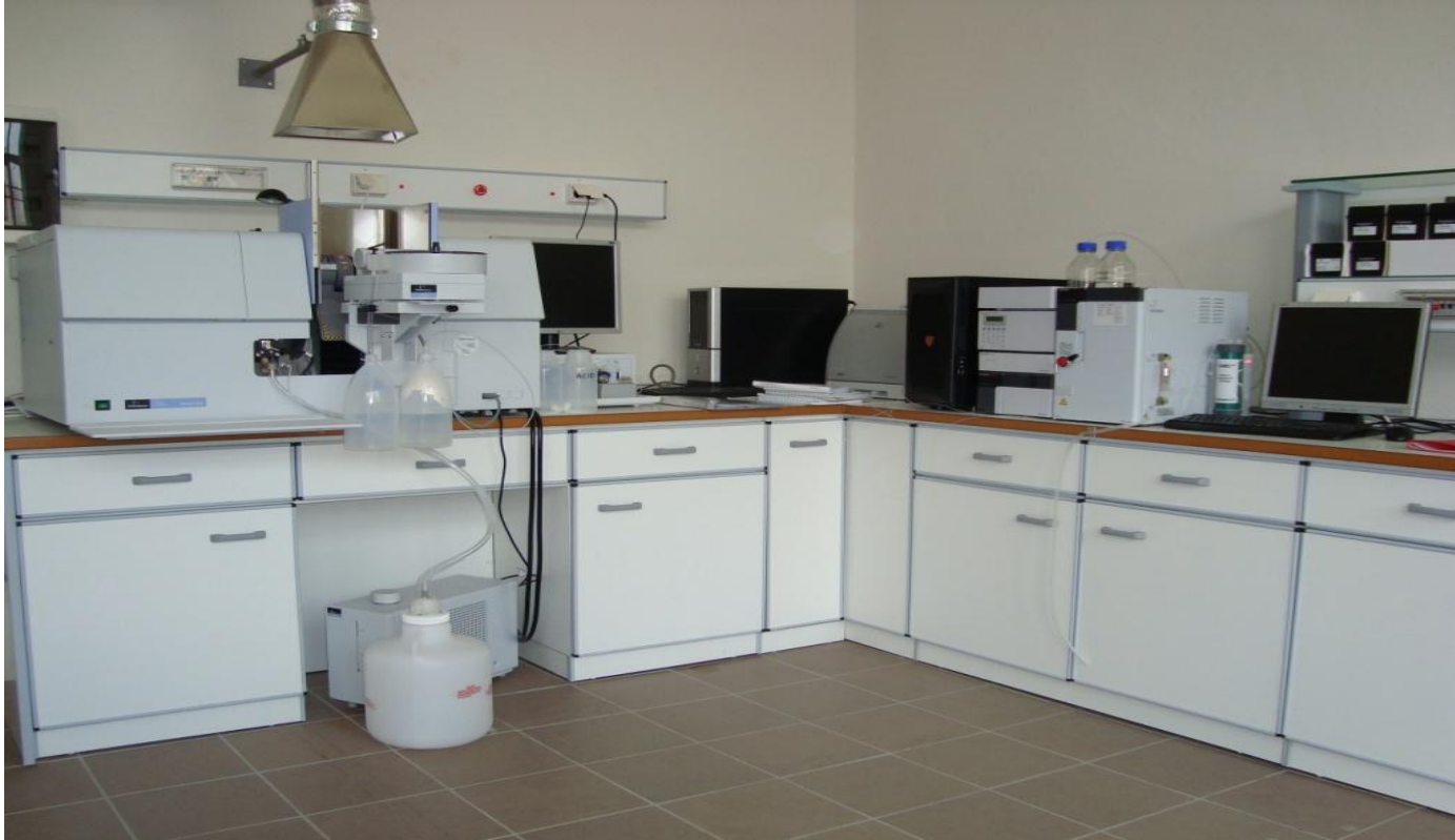
Atomic Absorption Spectrometer A Analyst 800 of Perkin Elmer and Ion Chromatograph LC 20 AD of Shimadzu
